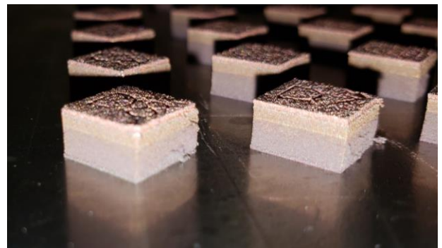
Figure 31: Visible layers after cleanup
