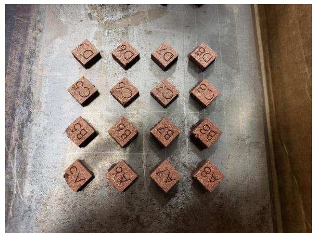
Figure 32: Parts after extraction. Notice rough surface texture.
